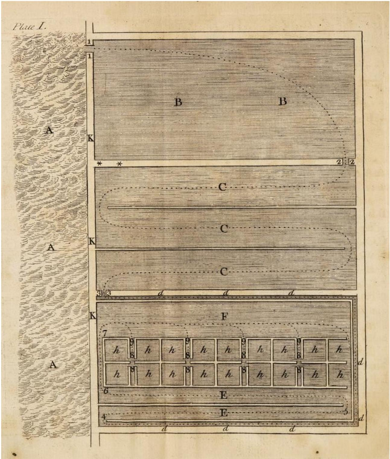
Figure 3. Plan of sun pans as used in France in the early 1700s by Brownrigg<sup>4</sup>. A=sea; B= first receptacle, 20 inches deep; C= second receptacle, 10 inches deep; h=salt crystallisation chambers, each 15 by 14 feet and no more than 1½ inches deep.
