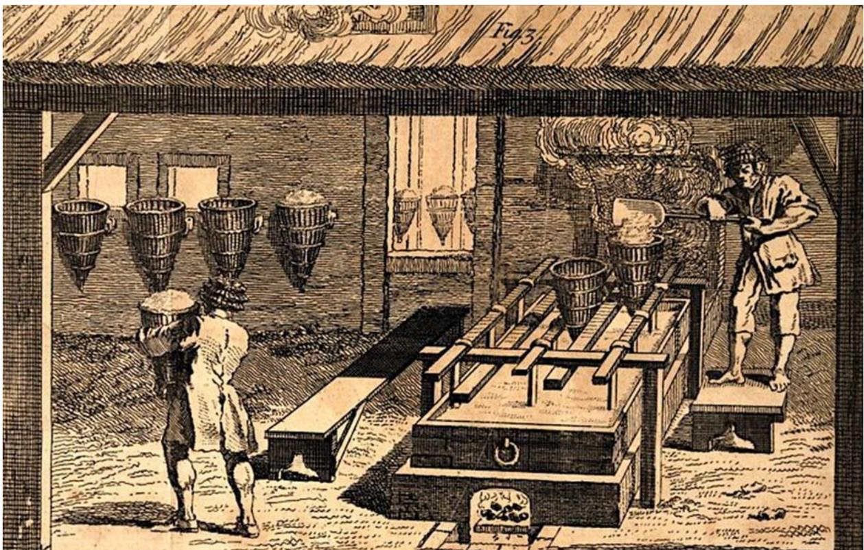
**Figure 4. A 16th Century saltworks (from Brownrigg<sup>4</sup>). This image shows the brine being heated and a worker scooping out the crystallising salt and placing it in wicker baskets to drain.**
